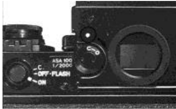
6. after deciding on the composition, turn the eyepiece shutter towards 'Close' setting
