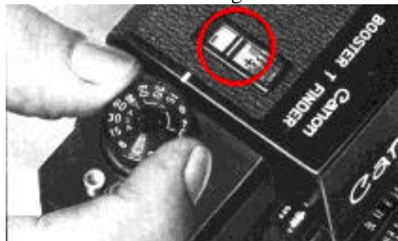
8. Turn the shutter dial or aperture ring to adjust the meter needle to the meter index
