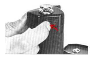
5. Remove the bottom cover of the body and attach the Motor Drive MF.
