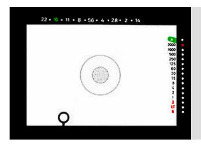
Viewfinder Display: 16-dot LED shutter speed display in-between speeds; Green shutter speed pointer overl and indicates shutter control dial setting on Manual Ap maximum aperture of the lens in use on the extreme rigreen figure; Exposure compensation tab appears who compensation pointer is set at any position other than '
