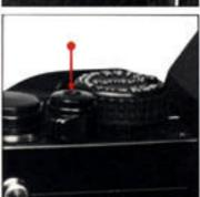
The LX self-timer provides a variable 4 to 10 second delay of the shutter release. Press the lever release button and turn the multi-f'unction lever counter-clockwise to set the timer delay. After making sure the shutter is cocked, press the shutter release button to activate the timer run. The timer can be cancelled before the start of its run by returning the lever to its original position. Once you press the shutter release button, it can no longer be cancelled.
