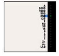
In the manual exposure mode your Pentax LX provides rapid response through-the-lens metering combined with an extensive manual shutter speed range from 1/2000th second to 4 full seconds. To set the LX for manual exposure control, press the shutter dial lock release and move the dial from the "Automatic" position. The shutter speed selected by the dial will be displayed in the camera viewfinder by a blue flag at the right-hand side of the scale.
