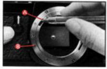
Super-Takumar and SMC Takumar screw-mount lenses can be attached to your Pentax LX by using the Pentax Mount Adaptor K. When using this accessory, however, the automatic diaphragm of the lens will no longer function and meter readings must be made with the lens apertuPe stopped down.
