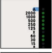
Green LEDs are used along the shutter speed scale between 1 /2000th and 1 /30th second to indicate hand-holdable speeds.
