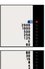
A red LED will glow next to the "A" index on the viewfinder scale to indicate overexposure. When this occurs, stop your lens down or change to manual exposure control to obtain acceptable exposures.
