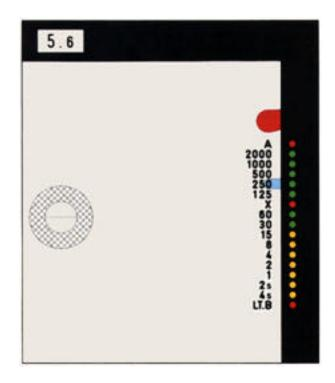
Aperture WindowDisplays f/stop set on camera lens.Red FlagExposure compensation warning.Blue FlagIndicates position of shutter dial.
