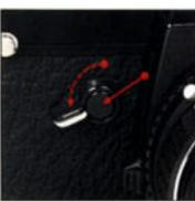
Your Pentax LX features a Multi-Function Lever which is used to operate the self-timer, preview depth of field and lock up the mirror. The lever operates as follows:
