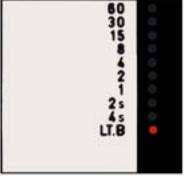
A red LED will glow next to the "LT, B" index on the scale when there is insufficient light for a proper exposure or when the camera has selected a time exposure longer than 4 seconds in the automatic mode.
