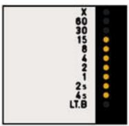
Yellow LEDs are used along the shutter speed scale between 1/1 5th second and 4 seconds as a slow speed warning and reminder to use a tripod or supplemental lighting, or to change the lens to a wider aperture setting.
