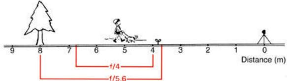
Depth of field is the area in acceptable sharpness in front of and behind the subject in focus at a particular f/stop setting. Depth of field can be checked visibly by activating the depth-of-field preview while looking through the camera viewfinder. If more precise information is required, however, the depth of field scales engraved on most camera lenses provide a convenient means of determining the approximate distances.
