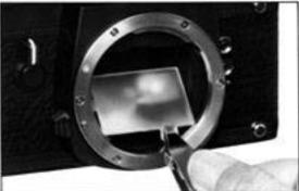
To change the LX Focusing Screen, use the pincette supplied with your new focusing screen. Insert the head of the pincette against the top plate of the mount so that the two ear-like tabs rest again,st the indentation in the plate as illustrated. Then, gently lift upward on the handle of the pincette until the focusing screen frame drops down.
